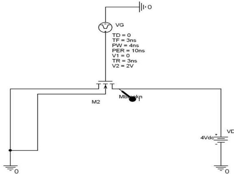
Figure :2 PSPICE schematic for transient characteristics
