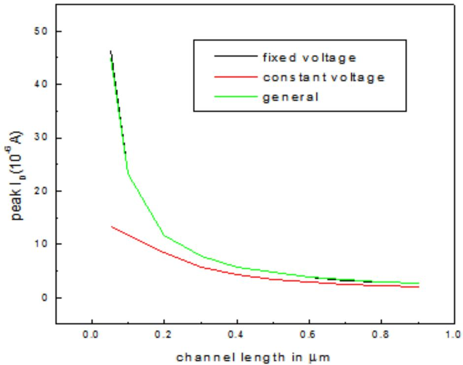
Figure 7. Rate of fall of  $I_D$  with the change in channel length for available scaling trends
