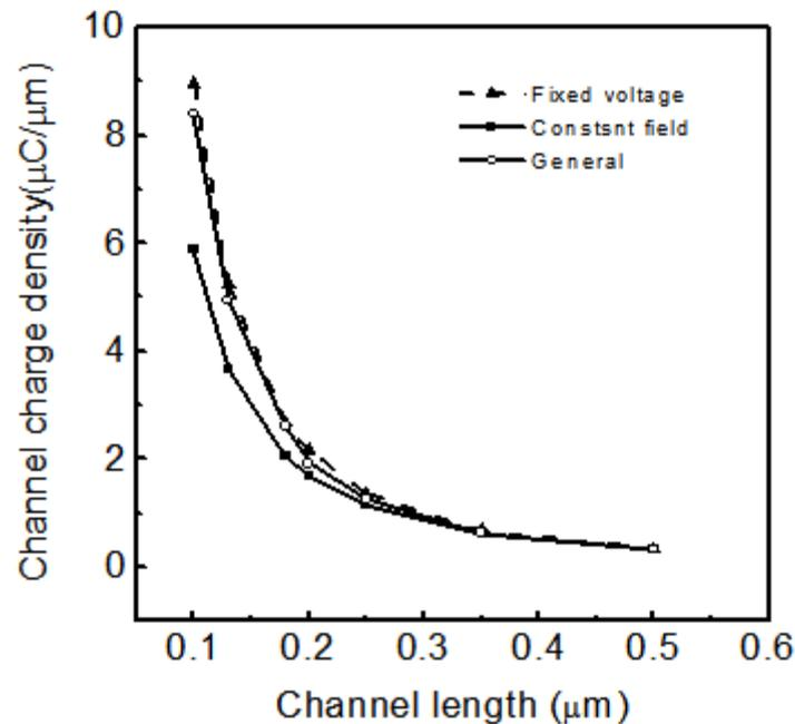
**Figure 1:** Linear channel charge density as a function of channel length for three types of scaling techniques
